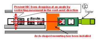
Measure to prevent HIC from dropping at an angle
