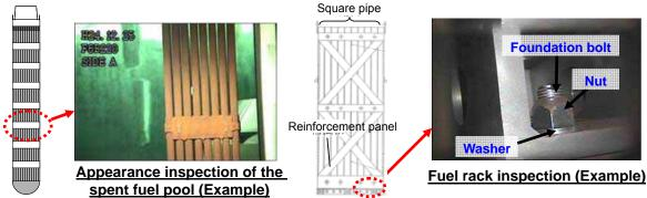
3. Inspection of the fuel, etc. in the common pool
