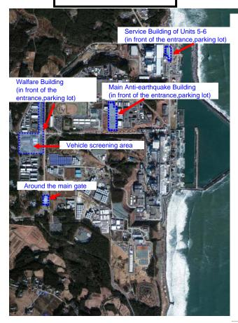
As the radioactive material concentration in air is below the level requiring mask (Particle Cs: 2x10<sup>-4</sup>Bq/cm<sup>3</sup>), the areas indicated in blue have been designated as area not requiring mask.
