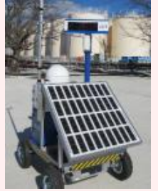
Installation of Dose-rate monitor
