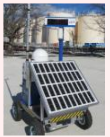
Installation of Dose-rate monitor
