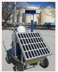
Installation of Dose-rate monitor
