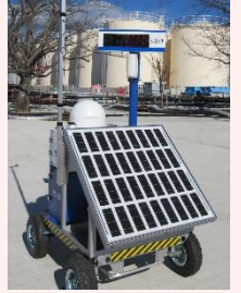
Installation of Dose-rate monitor
