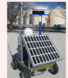
Installation of Dose-rate monitor
