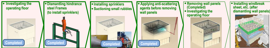
Flow of building cover dismantling
