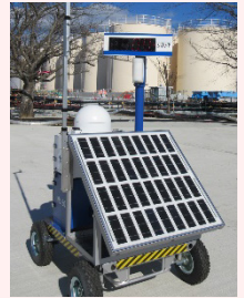
Installation of Dose-rate monitor
