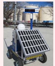
Installation of Dose-rate monitor
