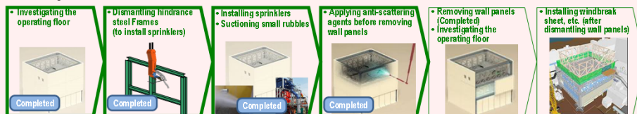
Flow of building cover dismantling
