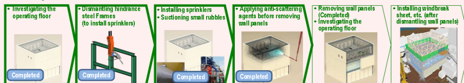
Flow of building cover dismantling
