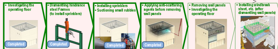
Flow of building cover dismantling
