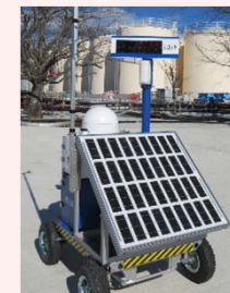
Installation of Dose-rate monitor
