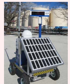
Installation of Dose-rate monitor
