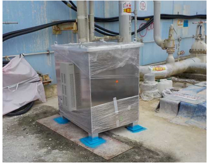
Figure 4: Muon measurement device (small device)
