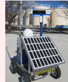
Installation of Dose-rate monitor
