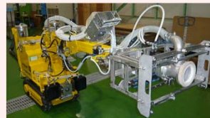
High-pressure water decontamination equipment
