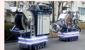
Dry ice blast decontamination equipment
