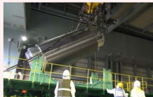
Loading the transportation container onto the trailer
