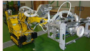
High-pressure water decontamination equipment
