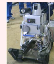
Robot for investigating the contamination status (gamma camera mounted)
