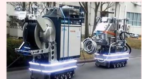
Dry ice blast decontamination equipment
