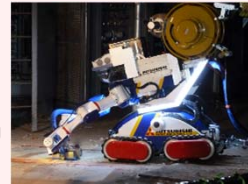
Aspiration and blast decontamination equipment
