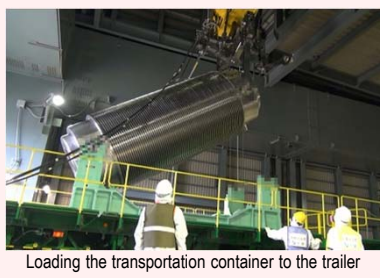
Loading the transportation container to the trailer
