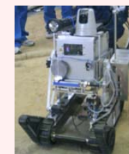
Robot for investigating contamination status (gamma camera mounted)
