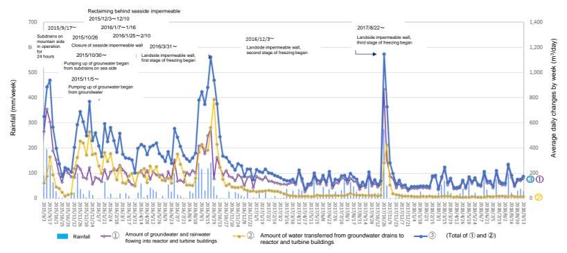
Amount of water transferred from groundwater drains to reactor and turbine buildings
