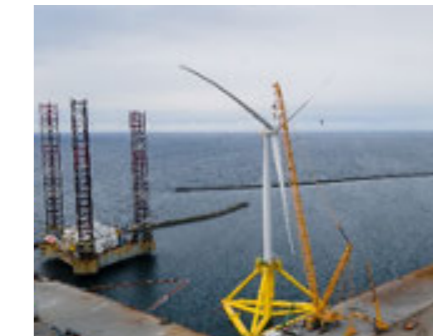
TetraSpar Floating Offshore Wind Turbine Demonstration Project The TetraSpar was designed and developed with the intention of industrialization, and it is expected to reduce the costs of float manufacturing, assembly and installation. TEPCO has participated in this project underway in Denmark and Norway since February 2021 and we are aiming for the early establishment of this technology.
