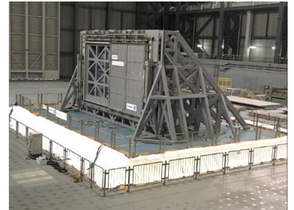
Blowout panels vibration test
