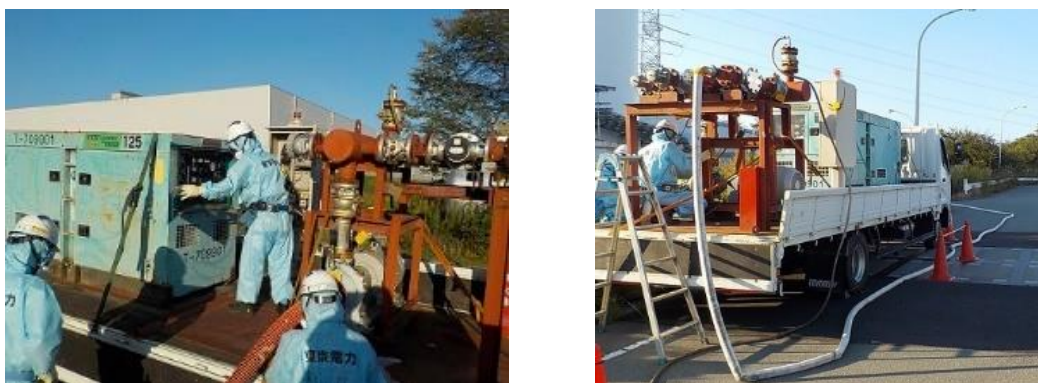
Spent fuel pool cooling water injection training (left; truck-based pump operation, right; sending cooling water)
