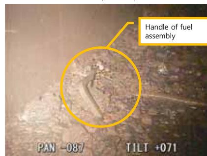
Deposits and parts of fuel assemblies observed during internal investigation of Unit 2 PCV (Jan. 19)
