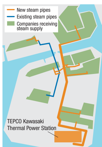
Overview of the steam supply business
