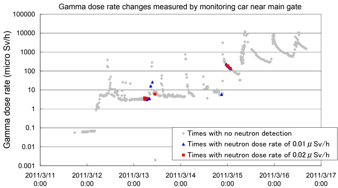
Figure 5 Gamma dose rates near the main gate
