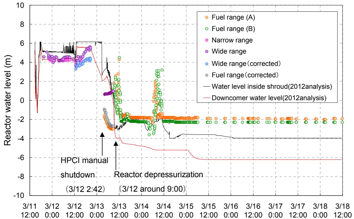
Figure 3 Reactor water level changes in Unit 3
