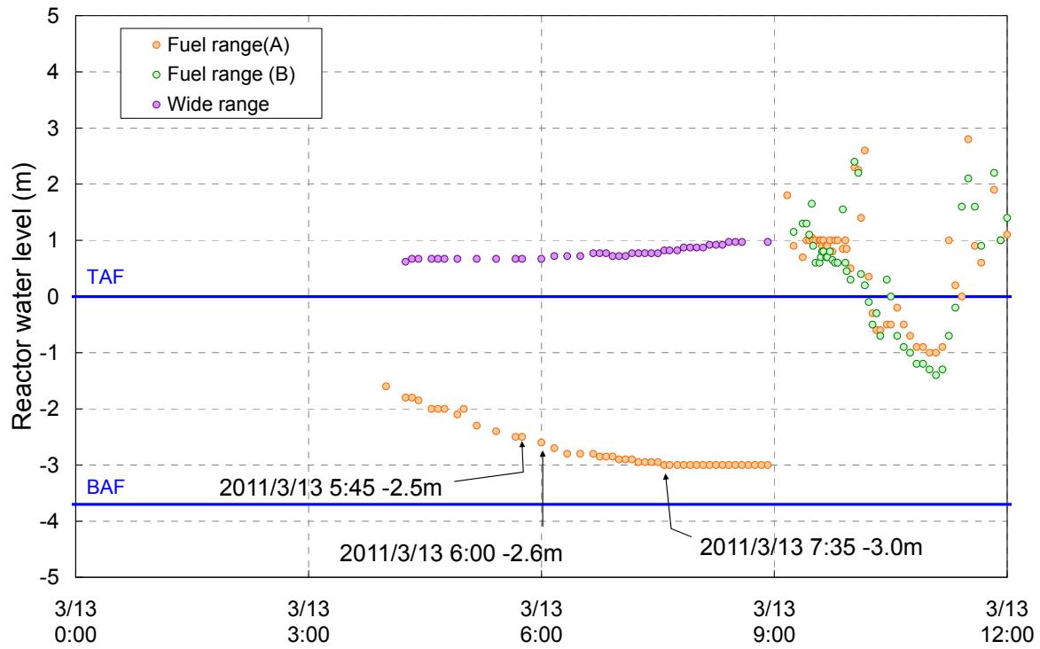
Figure 4 Reactor water changes in detail in Unit-3
