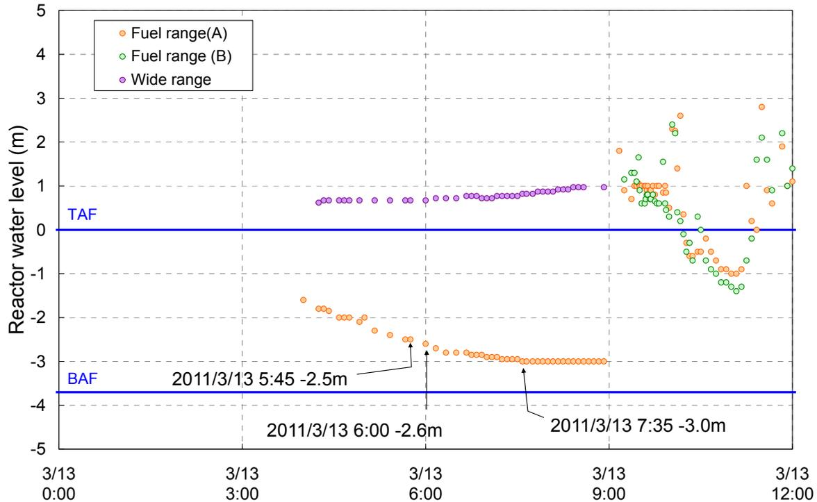
Figure 4 Reactor water changes in detail in Unit-3
