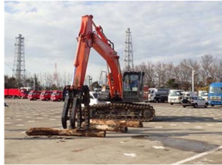
Training on picking up debris with the claw attachment (Kashiwazaki-Kariwa)
