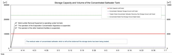
Note - The amount of water treated through the 2nd Cesium Adsorption Apparatus is estimated to be 780m<sup>3</sup>/d (Subject to change depending on the factors such as the levels of water accumulated in T/Bs.)
