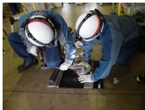
Directly managing disassembly and inspection of a valve
