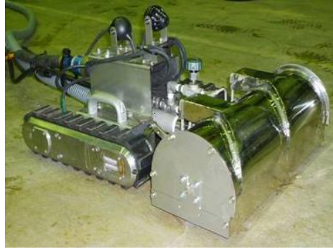
The remote decontamination equipment RACCOON with a brush head
