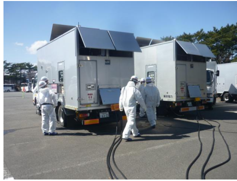
Loaded power supply car training at Fukushima Daini. (Left: Measurement of cable insulation resistance and connection to load car. Right: Parallel operation of power supply cars.)
