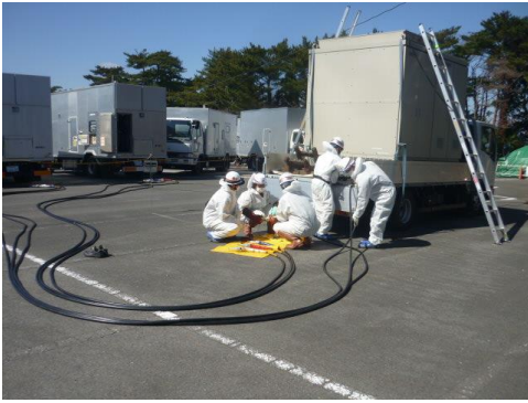
Loaded power supply car training at Fukushima Daini. (Left: Measurement of cable insulation resistance and connection to load car. Right: Parallel operation of power supply cars.)
