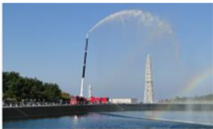
Deploying a water cannon truck intended for the use at higher locations
