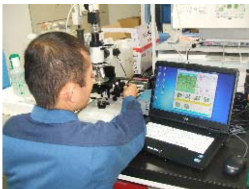
Lubricant diagnosis (quantitative ferrography analysis)
