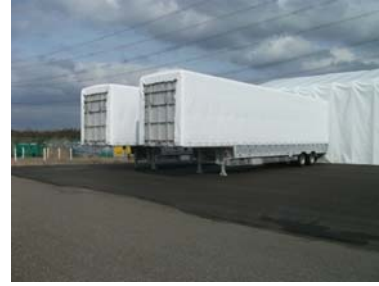
Deployment of trailers loaded with materials and tools to shorten installation time of stand-by heat exchanger (Kashiwazaki Kariwa)
