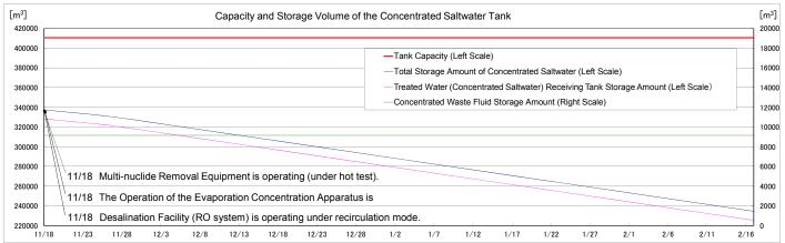
The treated water volume is assumed to be 780m³/d (Subject to change depending on the level of water accumulated in T/B).
