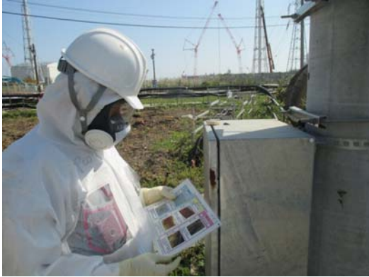
Use of a boundary sample of rust for electric installations (Fukushima Daiichi) (Patrol inspection)
