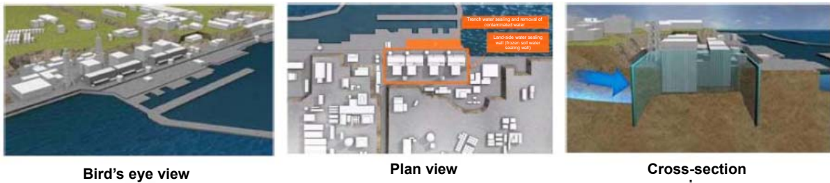
Overview of land-side water sealing wall work
