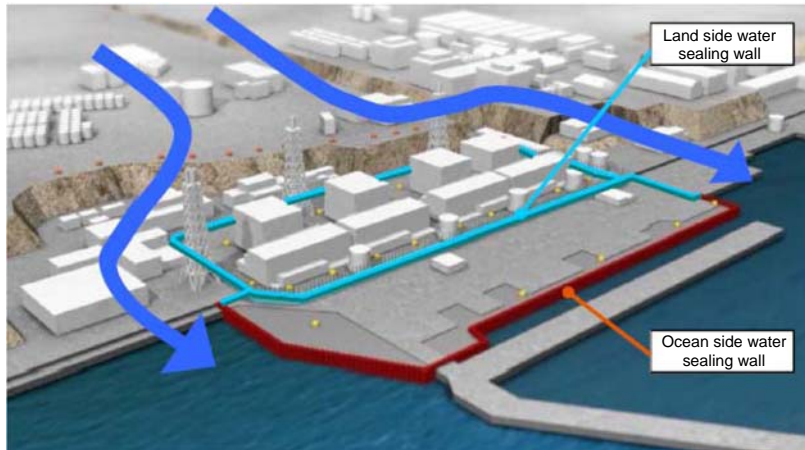
Flow of underground water after installation of frozen soil water Sealing Walls
