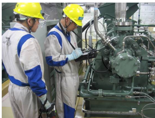
Collection of data directly by operators (e.g.: vibration diagnosis)
