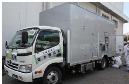
Power source vehicle : Power generation capacity (500kVA) is equivalent to power consumption of approx. 160 households.
