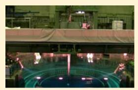
Hanging the fuel grab machine down into the reactor
