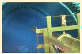
Fuel assembly being moved into the spent fuel pool (1)
