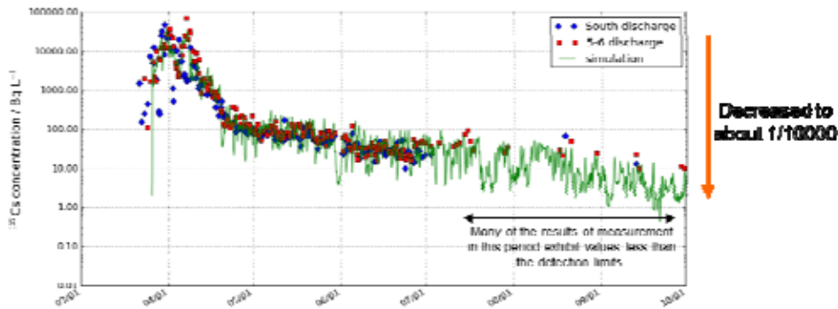
Figure 3 Concentration of radioactive materials in seawater near the water discharge canals of the Fukushima Daiichi Nuclear Power Station
