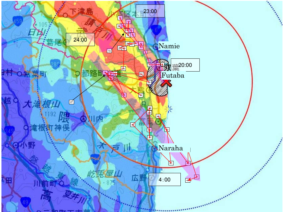
Figure 34. Path of Plume Released during Unit 2 Building Release after 20:00 on March 15
