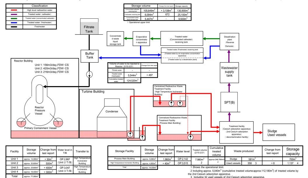
(Water transfer from Unit 2 to High Temperature Incinerator Building is planned. The transfer from Unit 3 to temporarily suspended, and after the resume, it is planned to transfer to Process Main Building.)
