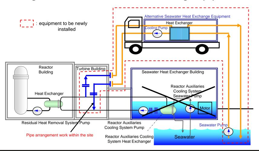
We have installed measures against inundation to seawater heat exchanger building by tsunami such as deploying fire-engines, alternative seawater pumps, spare motors for seawater pumps, etc. In addition to them, for more safety measures, we will install alternative seawater heat exchange equipment to cool the reactor and fuel pools.
