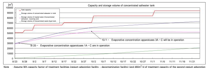
Assume 90% capacity factor of treatment facilities (cesium adsorption facility - decontamination facility) (and 480m³/d of treatment capacity of the second cesium adsorption
