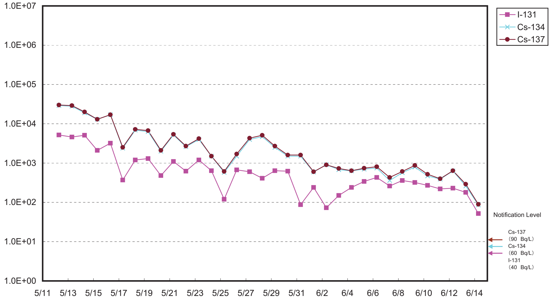
Radioactivity Density of Seawater around the Bar Screen of Unit 4 of Fukushima Daiichi NPS (outside the Silt Fence) (Bq/ L)
