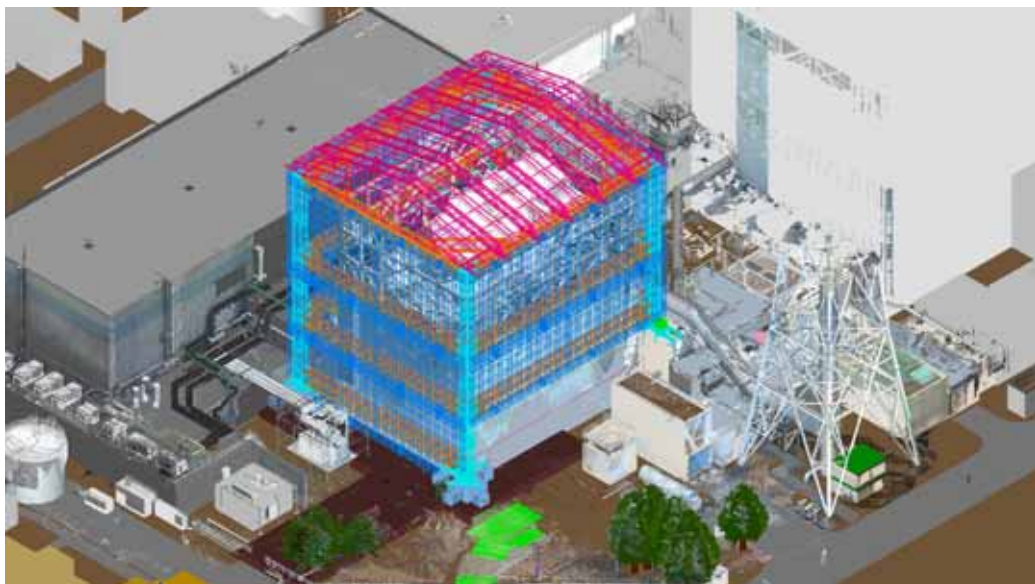
( b ) Composite image of polygon data converted from point group and 3D building CAD data.
