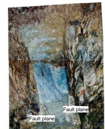
Sketch · photo of fault outcrops (Loc.T365) : Fault with granodiorite and Futaba group Ashiba formation rudaceous grit stone side by side. The part approx. 1m in between the two surfaces is soft clayish fractured part.
