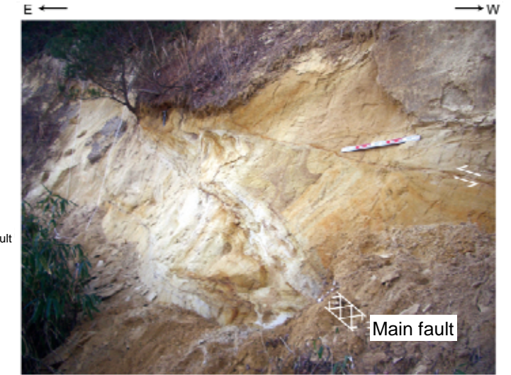
Loc.Y531 ( Washiashi, Yamamoto town ) : reverse fault at Tomioka fault. The fault surface conglutinated and merged into surrounding rocks.
