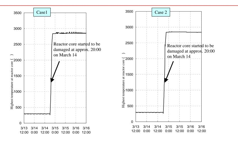
· After the drawdown, temperature at reactor core rose and it starts to be damaged in both cases.
