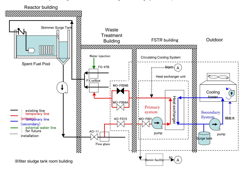
Summary drawing of the alternative cooling and filtering system of Spent Fuel Pool Attachment 2
