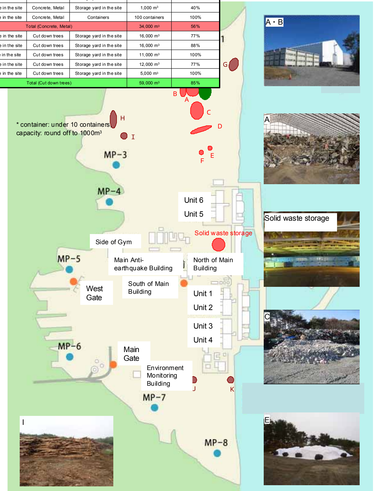
Fig. 2 Management of rubble and cut down trees
