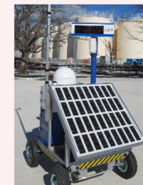
Installation of Dose-rate monitor
