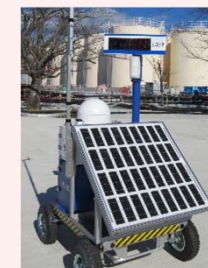
Installation of Dose-rate monitor
