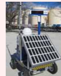
Installation of Dose-rate monitor
