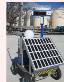
Installation of Dose-rate monitor
