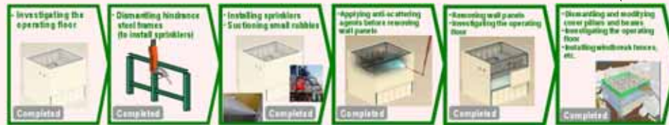
Flow of building cover dismantling (the latest status)
