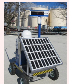
Installation of Dose-rate monitor
